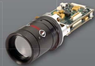
Analog configuration with 28° f/1.2 lens
