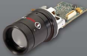
Digital configuration with 28° f/1.2 lens
